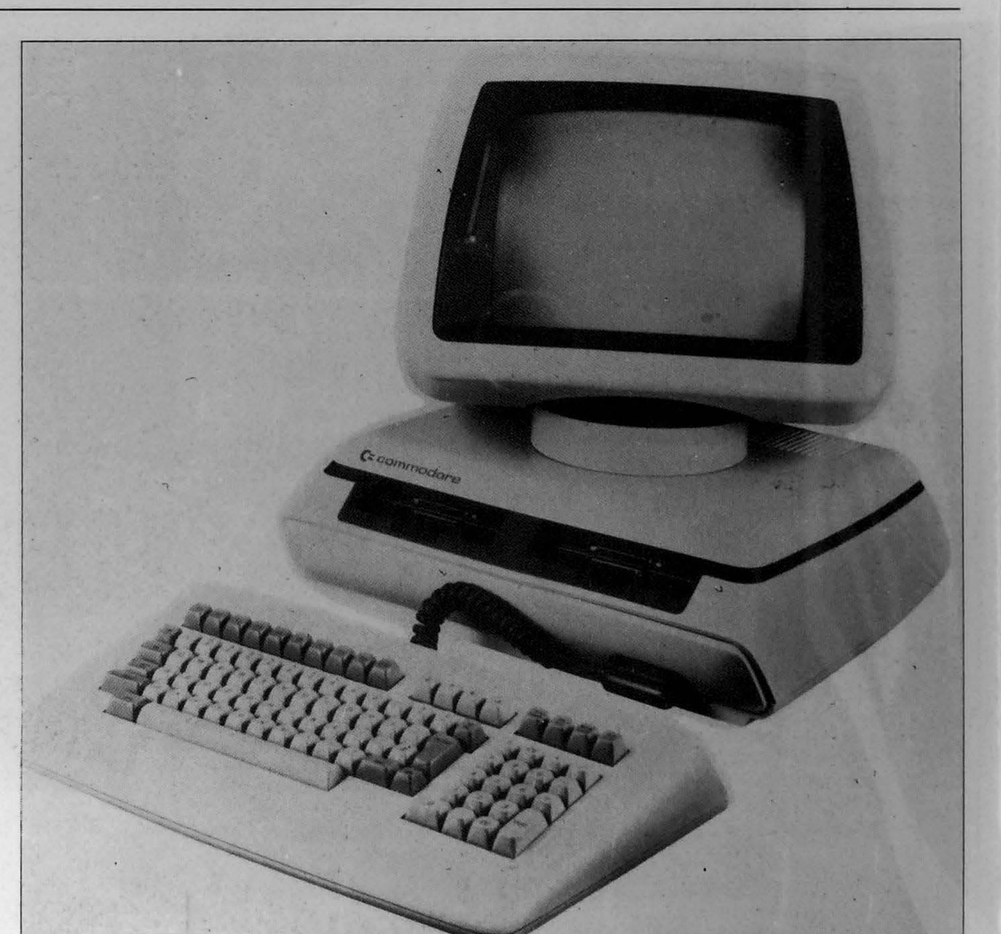
**CPU**: 6509, 1MHz **Ram:** 128-896K **Rom:** 28K Keyboard: Full, 94 keys **Display type:** TV or Monitor, colour Display ability: 40x25 text, 320x200 graphics Sound: 3 voices with special effects, external Storage: Own cassette recorder £45, optional disks up to 2x1Mb floppy plus 5Mb hard disk Interfaces: RS232, IEEE, User port, Joystick, Expansion connector
