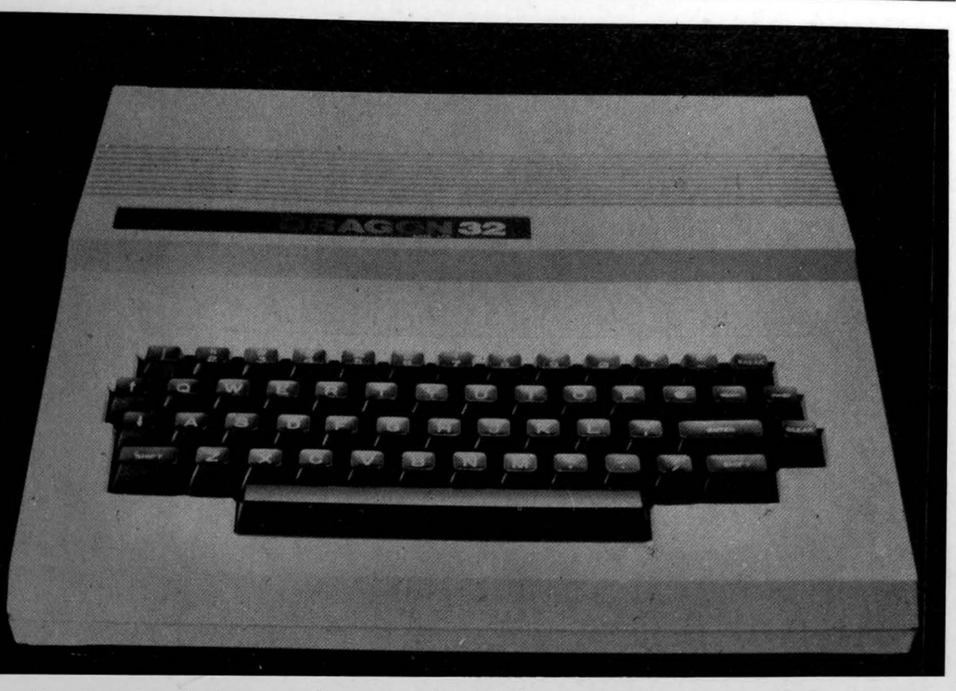
CPU: 6809, 1Mhz Ram: 32-64K Rom: 16K Keyboard: Full, 53 keys Display type: TV or Monitor, colour
