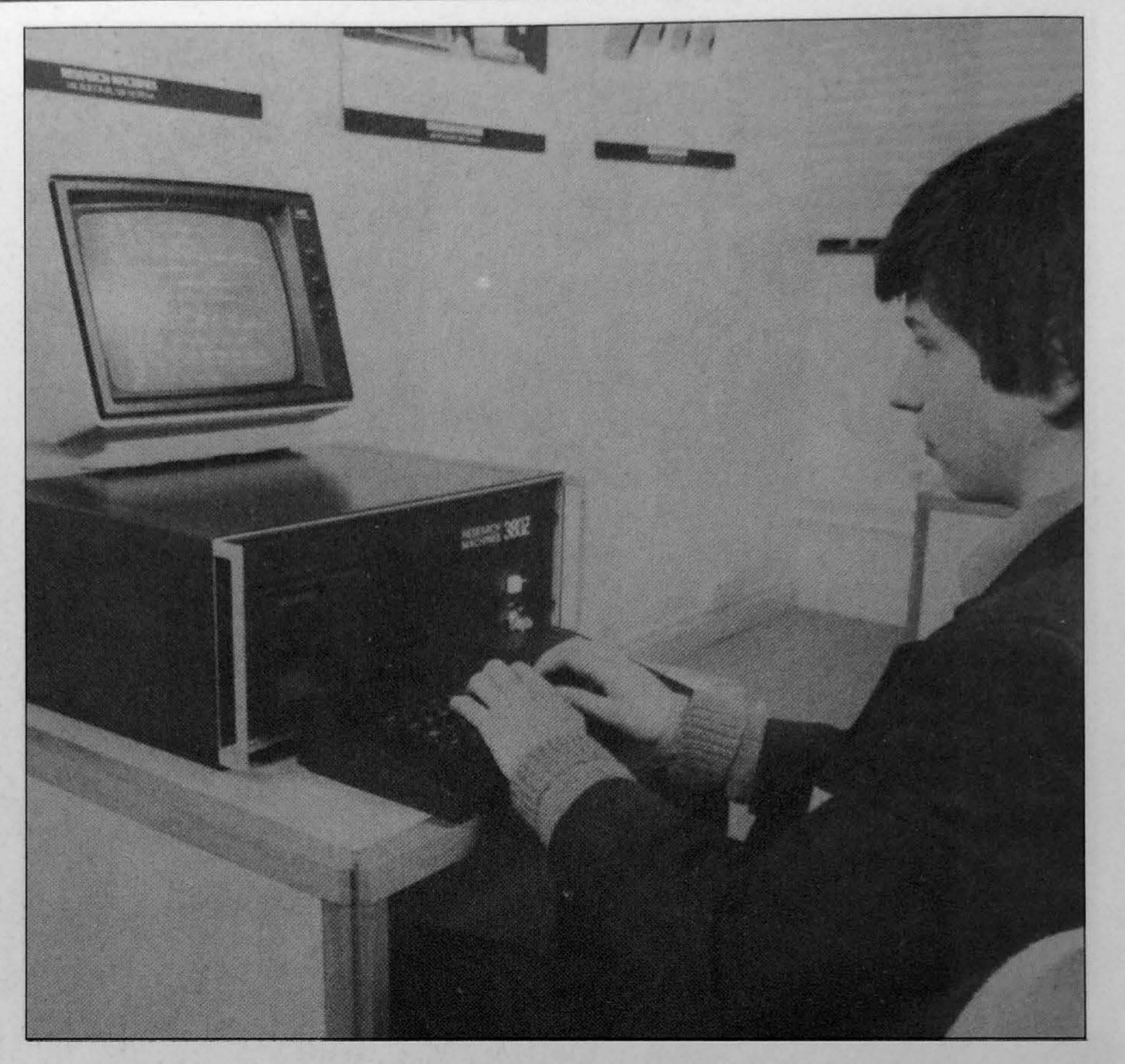
**CPU:** Z80, 4MHz **Ram:** 32-56K Rom: 4K Keyboard: Full, 65 keys Display type: TV or Monitor, optional colour Display ability: 40x24 text, optional 80x24 text, 320x192 graphics, choice from 256 shades/intensities Sound: None Storage: 2x144K floppy, optional 2x241K 8 inch floppy Interfaces: RS232, Parallel, **IEEE488** Languages: Basic, optional Fortran, Algol, Logo Operating system: CP/M Software included: None Software availability: Good Guide price: £1900
