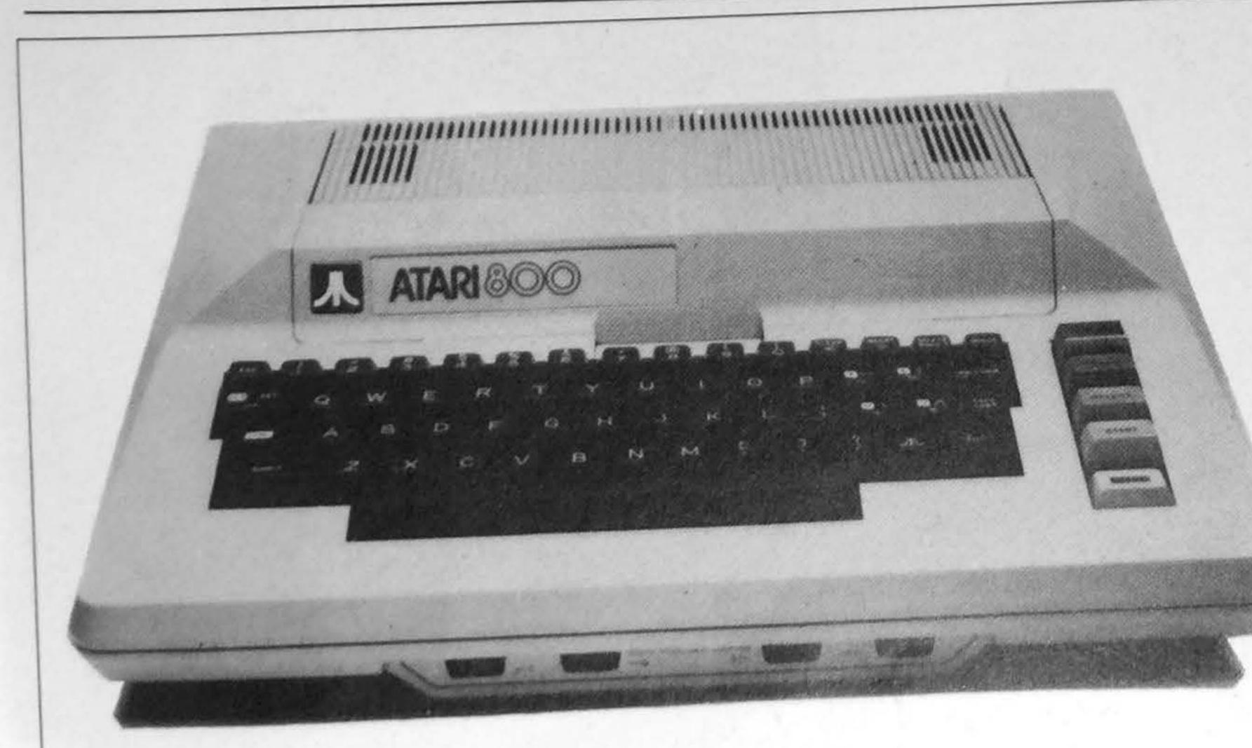
**CPU:** 6502, 1.8MHz **Ram:** 48K Rom: 10K Keyboard: Full, 61 keys Display type: TV or Monitor, colour Display ability: Up to 40x24 text, up to 320x192 graphics, choice from 256 shades/ intensities Sound: 4 voices with special effects, external Storage: Cartridges, own cassette recorder £50, up to 4x88K floppy Interfaces: 4x joystick, interface for disks, printer and cassette recorder, optional RS232 and Centronics Languages: Basic, optional
