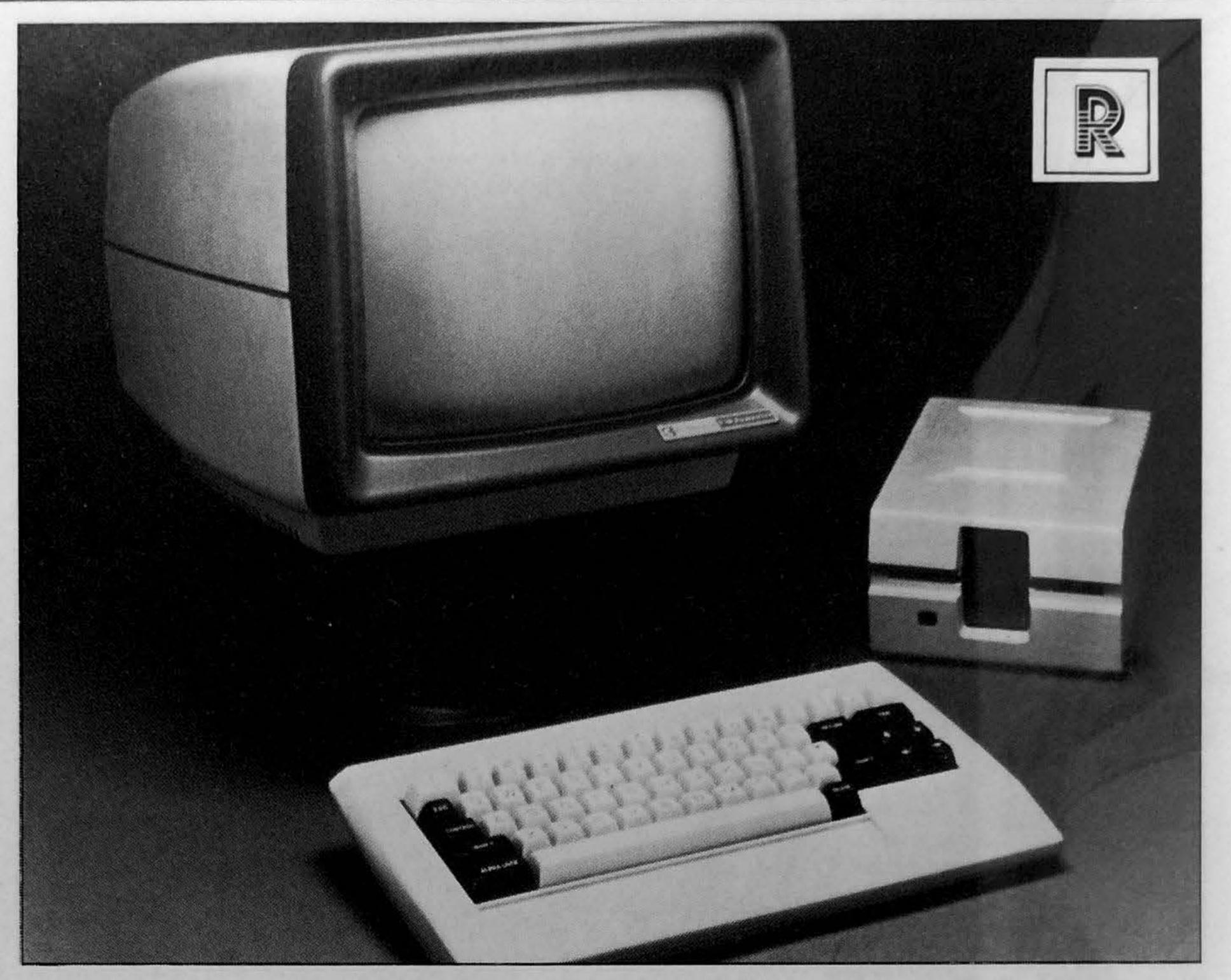
CPU: Z80, 4MHz Ram: 64K Rom: 24K Keyboard: Full, 59 keys Display type: Built in 12 inch monitor, monochrome Display ability: 80x25 text, some graphics characters Sound: Beeper
