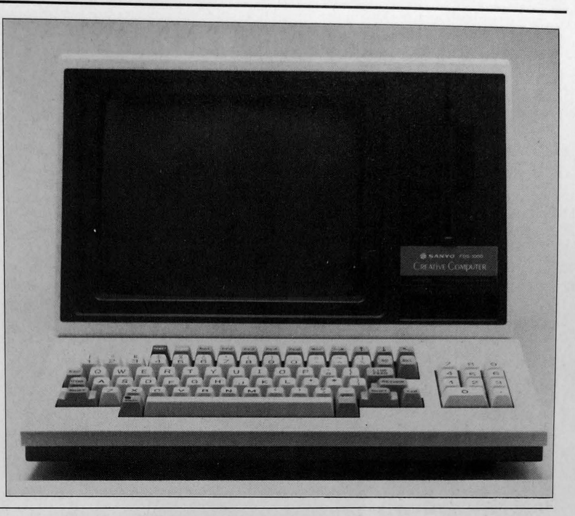
Display type: Built in 12 inch monitor, monochrome Display ability: 80x25 text Sound: Notes, internal speaker Storage: 1x320K floppy, optional 3x320K floppy Interfaces: RS232, Centronics Languages: Basic Operating system: CP/M Software included: Demonstration Software availability: Very good
