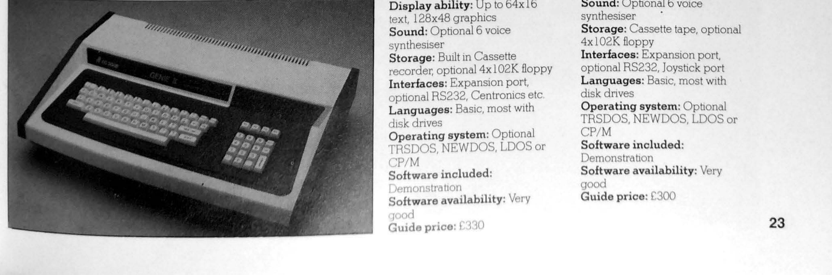
CPU: Z80, 1.7MHz Ram: 16-48K Rom: 13K Keyboard: Full, 54 keys Display type: TV or Monitor, monochrome Display ability: Up to 64x16
